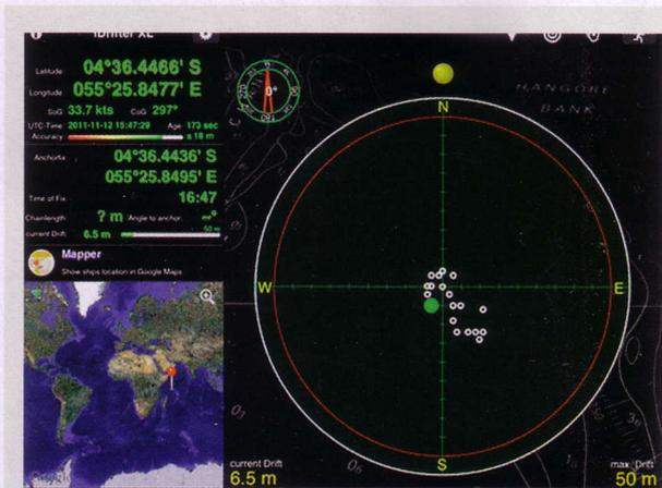
iDrifter screen showing position of anchored yacht as it swings
