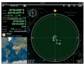
The iPad App, iDrifter XL, serves to continuously monitor your vessel's GPS position when anchored. The program displays the current drift of the yacht relating to the anchor - selectable either as a radar-style screen or as a map in Google Maps.
